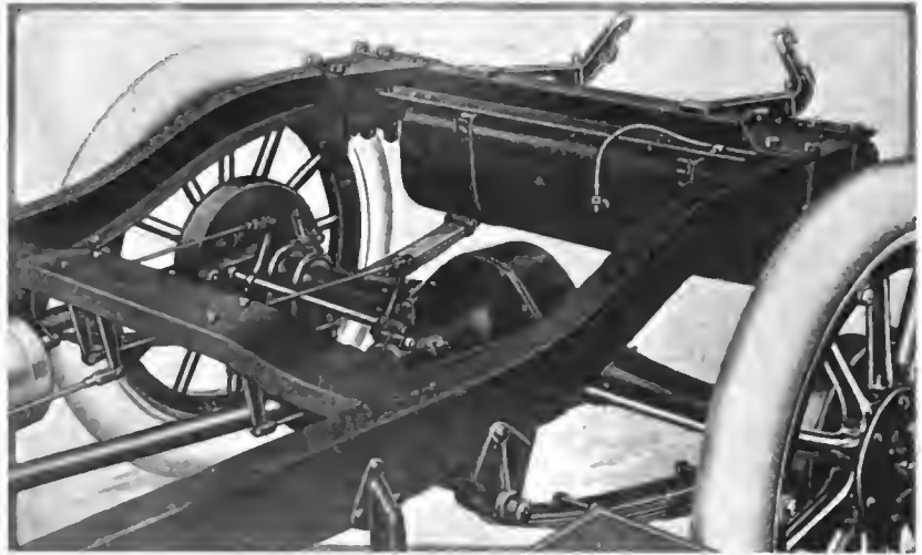
Rear end of Velle chassis, showing brake balance gear
